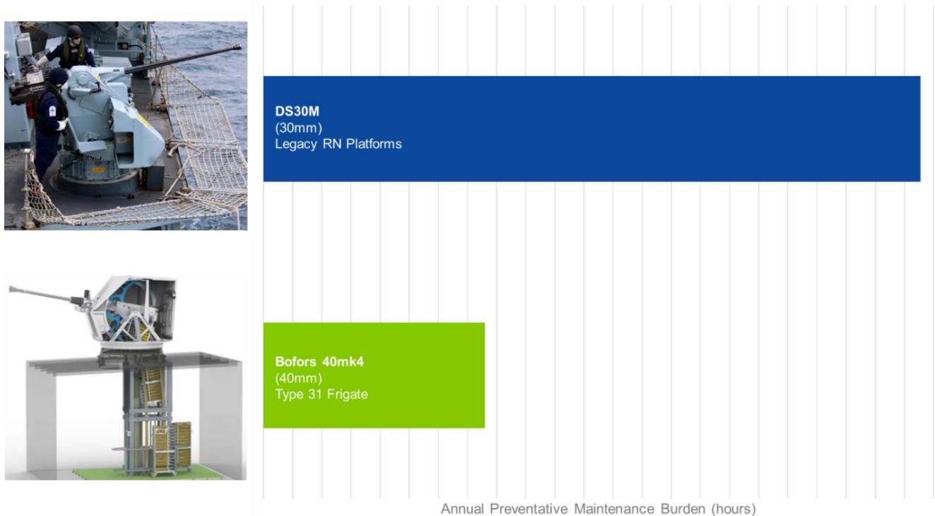
Figure 8. Type 31 annual preventative maintenance burden example (BAE Systems Bofors 40mk4), shown as a comparison to legacy RN equipment (data extracted from RN Unit Maintenance Management System (UMMS); axis scale redacted).
